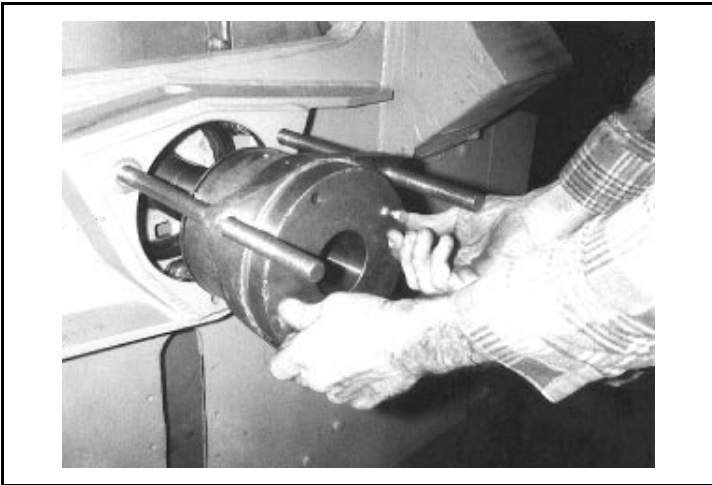
FIGURE 7 (MSSM0303AE) Installing the Bearing Housing Setting Fixture onto Housing (42" machine shown)
