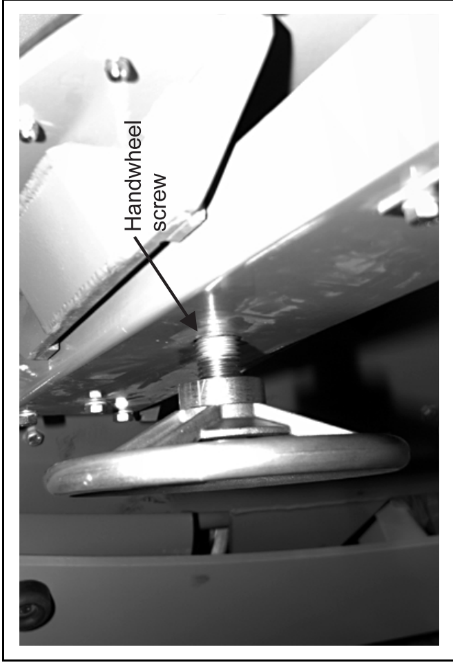
FIGURE 14 (MSSM0201CE) Handwheel Screw (42" Divided Cylinder and Staph-Guard® only)
